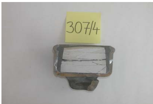
Figure 13. Critical crack growth – the tensile strength of the insulator was less than 80 kN
