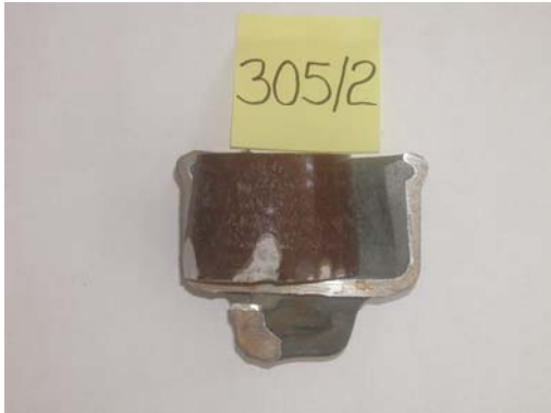
Figure 10. Damages of the edge of insulator
